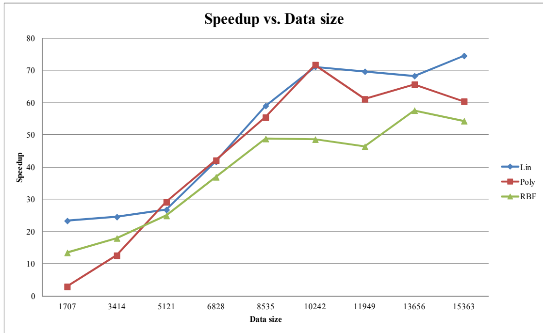
Figure 3.19: Embedded Hardware for CO-Based SVM: Speedup vs. Data Size for Cancer Benchmark Dataset
